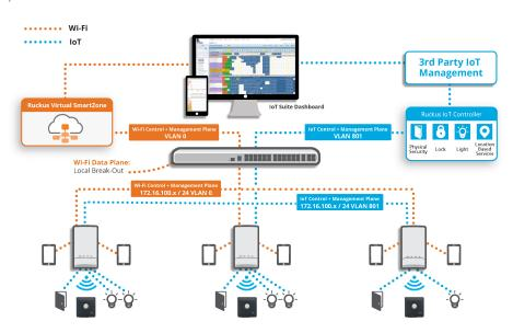
Once a worker activates the panic button, the REACT Mobile system tracks them as they move throughout the property, providing updated room or location information in real-time. At the same time, the versatile RUCKUS IoT Suite can trigger security cameras, lighting, door locks, and other connected systems to activate as part of the response. You can also use the IoT Suite to generate additional notifications to key responders, including SMS messages, E911 notifications, and emails.
