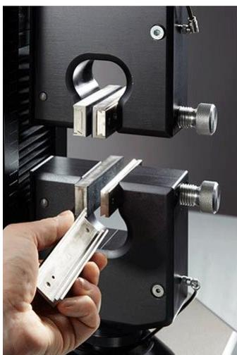
The grip is secured onto the base of Titan with the use of a tooling adapter.
