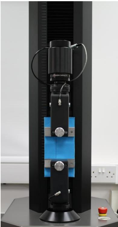
Specimen in the jaws ready for testing
