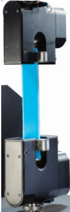
These grips are heavy. When changing the grips, it is recommended that the top beam is lowered so that the grip is at a manageable height.
