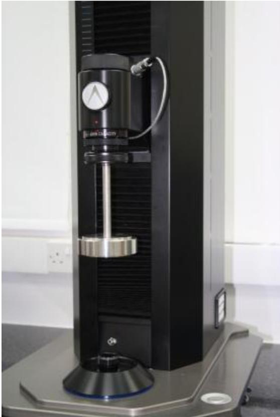
One at a time, carefully place all 5 circular check weights on to the Check Weight Holder, ensuring they are mounted centrally.
