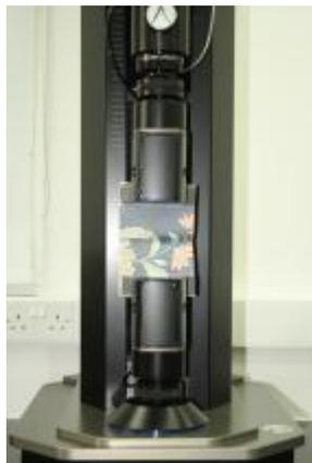
Secure the specimen in the jaws with the seam mid-way between and parallel to the edges of the jaws.
