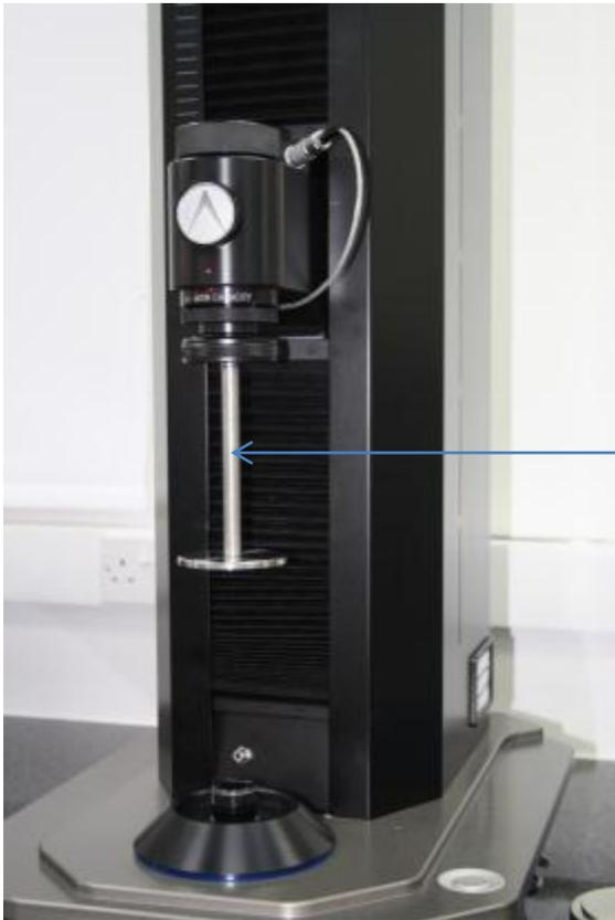
Remove both the top and bottom jaws from the screw thread adapter.
