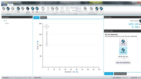
Using the Jog Down button (or Jog Up button if required), move the Top Jaw until the specimen can be gripped by the Bottom Jaw.
