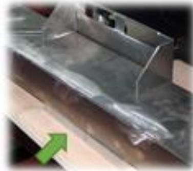
Remove the side frame and gently push on one side of the Instrument again to raise the feet to remove each of the Foot Supports
