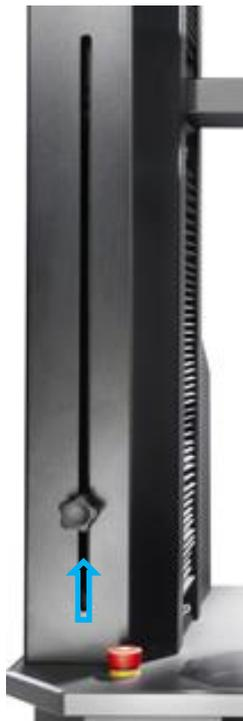
The crash protection must be set before a test is started. This prevents the jaws or tooling from crashing together and damaging the load cell, grips or tooling.
