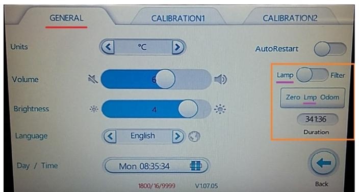
Note: the odometers are counter-up timers and no warnings are displayed when certain times have elapsed.
