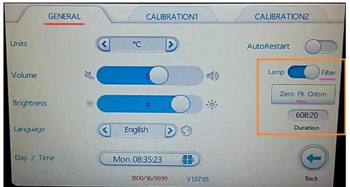
To view the Lamp odometer, move the toggle to "Lamp" – the duration in hours : minutes is displayed.
