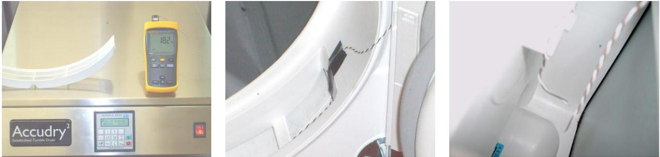
Figure 16: Locating the calibrated digital thermometer under the drum filter
