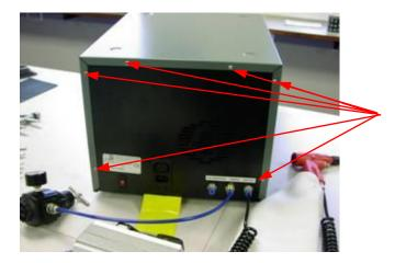
3) Slacken the 4 screws (2 each side) at the front of the unit.
