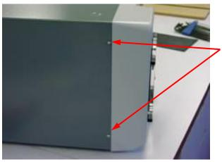
4) Pull the main cover towards the rear of the Impulse so that the front clamp bars disengage then remove the cover completely.
