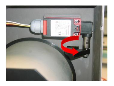
6) Refit the cover in the reverse order of the above and check the switch adjustment is still correct.
