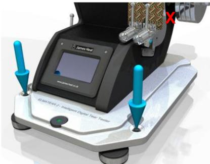
Press both of the Pendulum Switches at the same time to release the pendulum.
