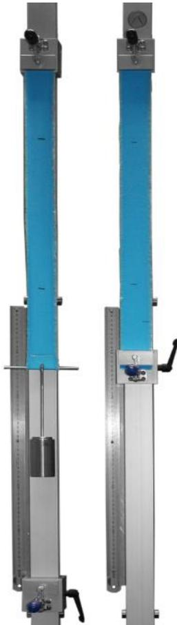
***ASTM D3107 - Stretch Properties of Fabrics Woven from Stretch Yarns*** consists of 2 parts - both of which are carried out on [FlexiFrame](#).
