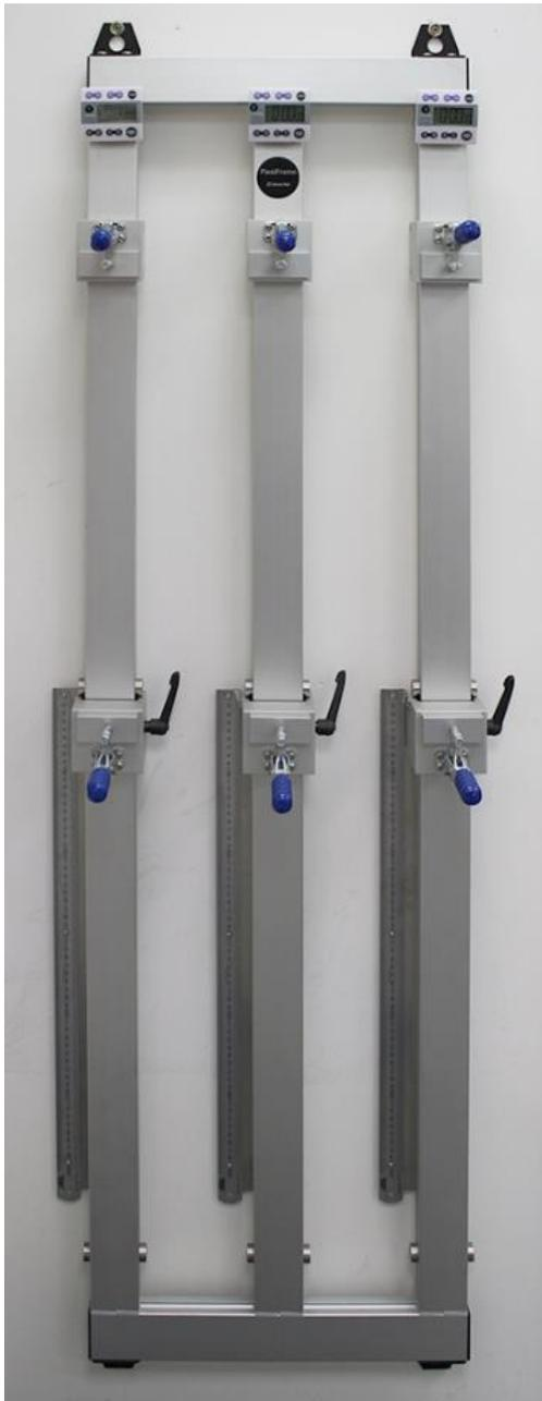
FlexiFrame is available as a 3 station ready assembled unit. This may be mounted on the wall using the 2 brackets attached to the top of the instrument.
