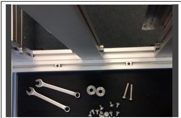
With the frames and base facing you, choose the frame which has the bottom left end cap removed. Locate this into the left hand side in the wheeled base. Push down firmly until the unit sits flush inside the bottom black clamp.
