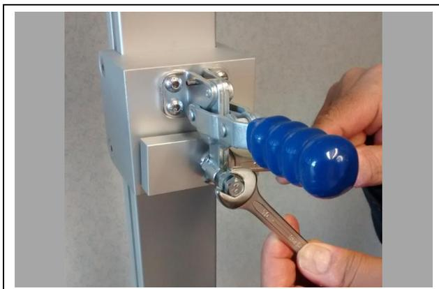
The top clamps are opened by lifting up the blue handle.
