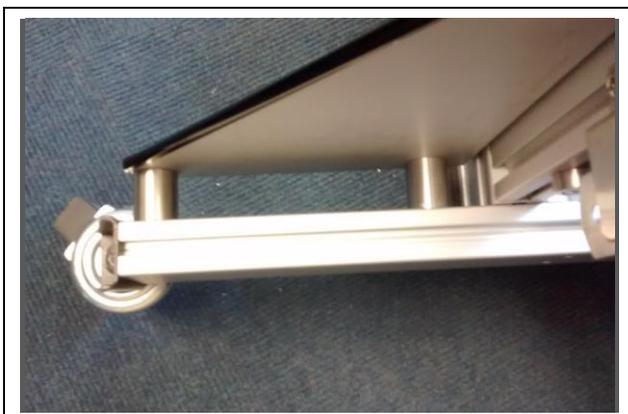
Space the left hand web away from the base using the spacers. Use the long screws and 5mm hex key to fasten onto the base.
