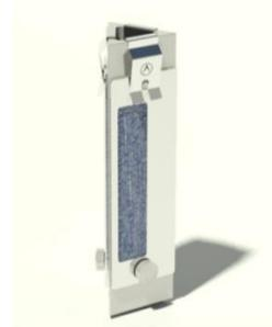
The holders can be fitted with an assortment of masks which allow the user to make comparisons between exposed and unexposed areas of the specimen and any control materials used:
