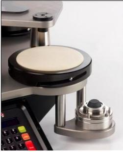
Place the hard rubber Precision Ball with the 20mm diameter end making contact with the specimen.
