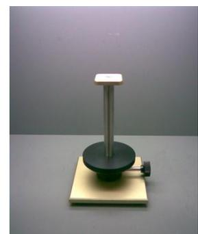
794-512 Specimen Mounting Device and 902-222 Sample Cutter 38mm
