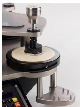
Place a loaded Sample Holder on each of the Abrading Tables.
