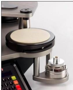
Place the Sample Holder Body on to the Sample Holder Nut and carefully engage the screw threads.
