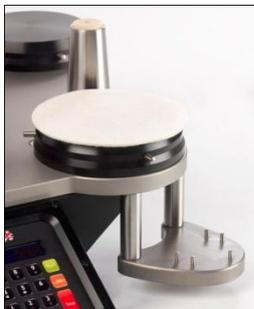
Place a 140mm diameter piece of Felt centrally on the Abrading Table.
