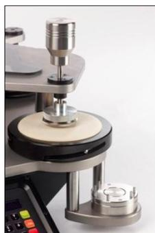
Mounted Sample Holder, complete with Spindle and Loading Weight.
