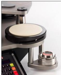
Place the Pinned Ring, needles first, down through the specimen into the holes in the modified Sample Holder Nut.
