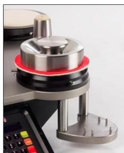
Carefully place the Pressing Weight centrally on to the Sample, taking care not to move Felt and Sample.
