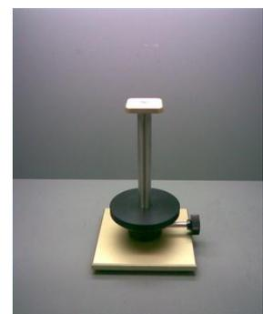
794-512 Specimen Mounting Device and 902-222 Sample Cutter 38mm
