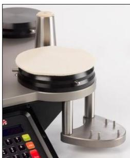
Place a 140mm diameter piece of SM25 Abrasive Cloth, face up, and centrally on the Felt.
