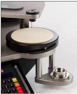
Carefully place the Sample Holder Insert in to the Specimen Holder Nut, on top of the PU Foam.
