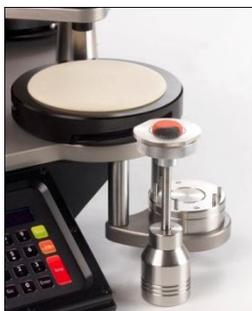
Check the specimen is securely held. Note how the specimen protrudes out of the Sample Holder Nut.
