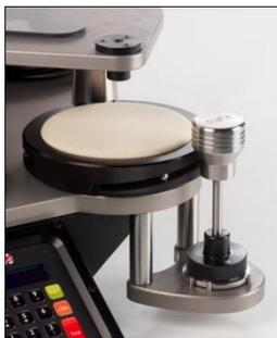
Check the specimen is securely held and none of its edge protrudes out of the Sample Holder Nut.
