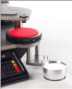
Place the Specimen face down on the Specimen Mounting Mandrel.
