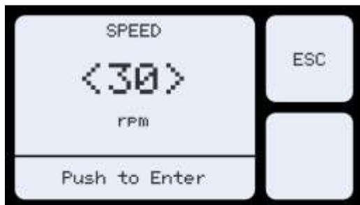
When the correct Speed is displayed, push the PR Selector to Enter the new value.
