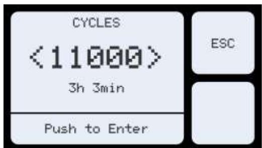
When the correct number of cycles (revolutions) is displayed, push the PR Selector to Enter the new value.
