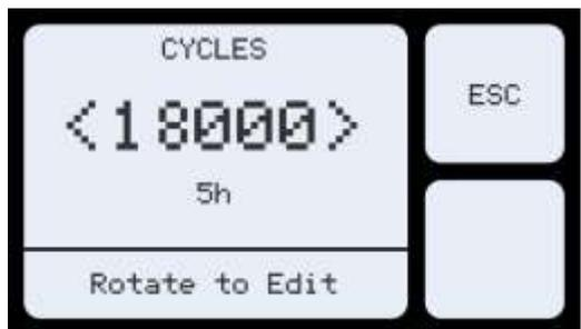
Rotate the PR Selector to change the number of cycles (revolutions) required.
