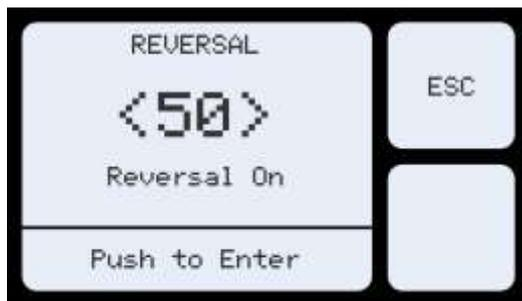
When the correct Reversal status is displayed, push the PR Selector to Enter the new value.
