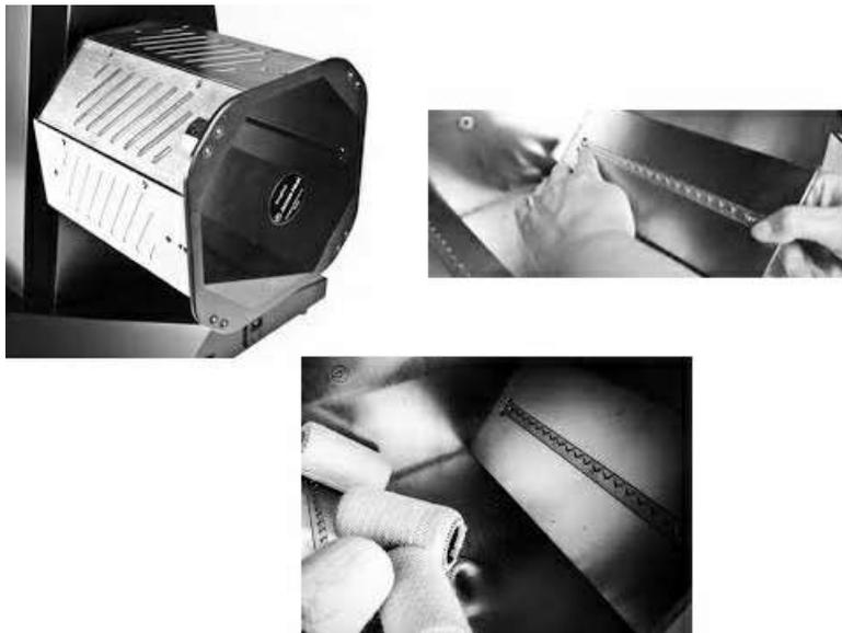
SnagPod: connected to Orbitor, pin bars specimens on tubes.
