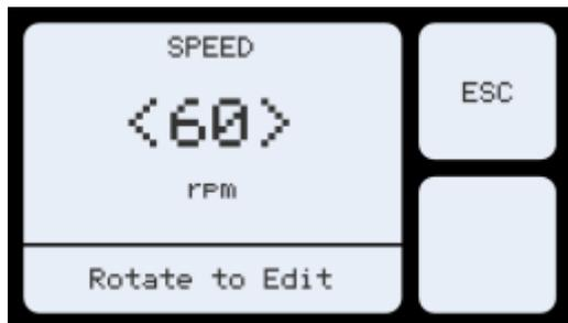
Rotate the PR Selector to change the Speed required.
