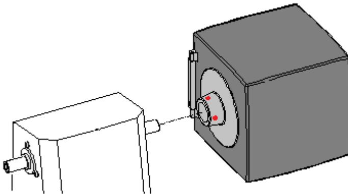
**NEVER** lift the machine by the test chambers. This will result in damage to the instrument.
