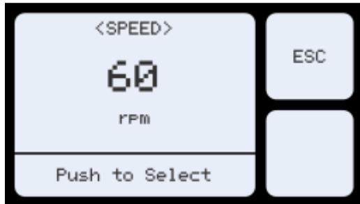
Orbitor<sup>2</sup> is capable of operating in several different speed modes, either 60rpm, 30rpm or 30rpm Reversing with a direction change after every 50 cycles (revolutions).
