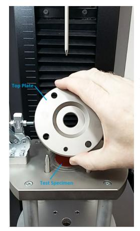
Remove the Top Plate and place the Test Specimen centrally over the bottom plate orifice, with the outer side of the glove facing upwards.
