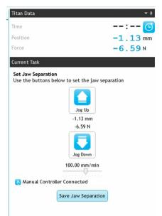
Carefully and slowly move the Nail Probe downwards until it just touches the surface of the Test Specimen.
