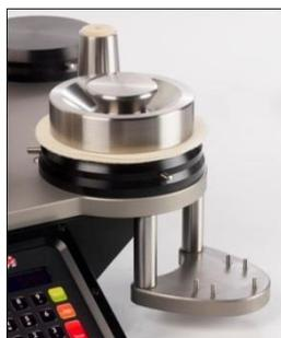
Carefully place the pressing weight centrally on to the SM25 abrasive cloth, taking care not to move felt and SM25 abrasive cloth.
