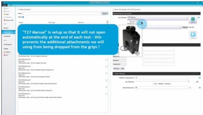
The "T27 Manual" Jaw Scheme is setup so that it will not open automatically at the end of each and therefore prevents the additional attachments from being released when opened
