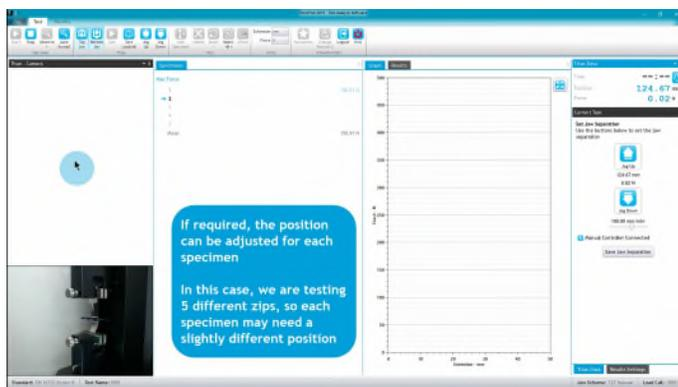
If required, the jaw separation position can be adjusted for each specimen
