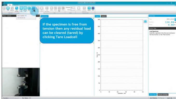
If the specimen is free from tension then any residual load can be cleared (tared) by clicking Tare Loadcell
