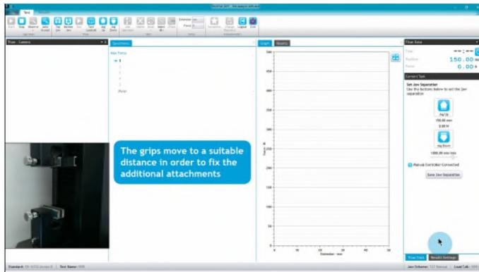
The jaws move to a suitable distance in order to fix the additional attachments
