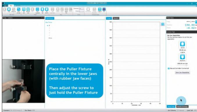
Place the Puller Fixture centrally in the lower jaws (with rubber jaw faces)
