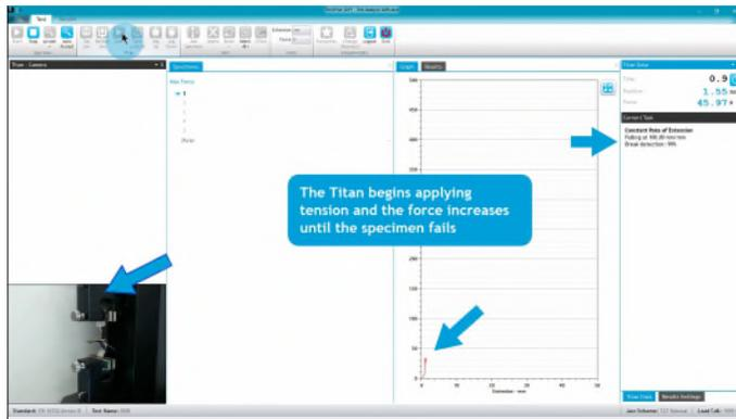
The Titan begins applying tension and the force increases until the specimen fails
