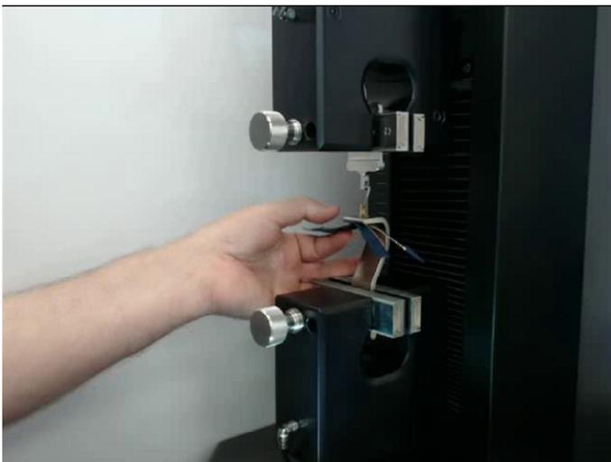
Insert the zip puller, from below, into the Puller Fixture
