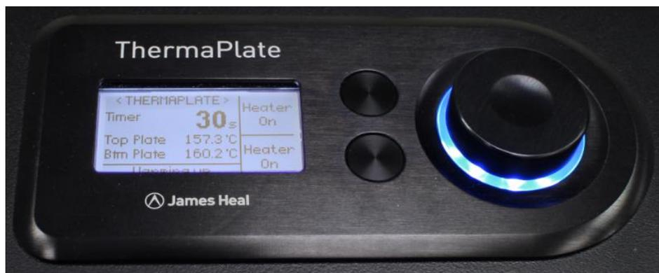
Set the timer to the required test duration by turning the selector button to <TIMER>. Select by pressing and then rotate to desired time. Press again to select and it will return to the home screen.
