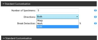
Standard Customisation can be used to change some aspects of the test such as the number of specimens tested (assumed to be the same number on both directions), which directions are tested, Break Detection.
