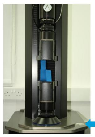
Position the specimen and close the **Top Jaw** and then the **Bottom Jaw**.
