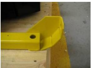
Before moving the instrument, remove the bolts (tools provided) which secure the Yellow Transport Frame to the wood pallet.
