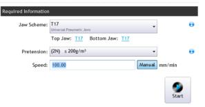
If a non-standard speed is required, click Manual and type in the required speed.
