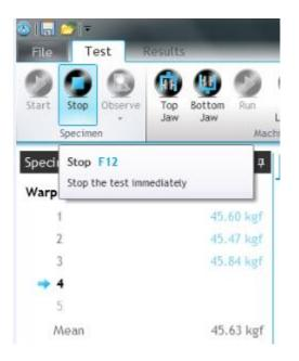
By default, the selected Standard requires 5 specimens to be tested in each direction.
