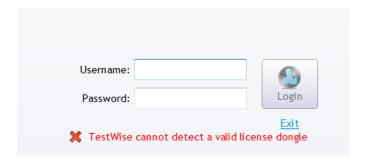
Whilst TestWise is running it also checks for the licensing dongle at random intervals. If the licensing dongle has been removed then the entire application is disabled. If the dongle is subsequently re-inserted it will take up to 5 seconds to be detected by TestWise and enable the interface.
