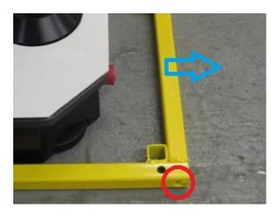
Once raised into the upright position, the bottom Yellow Transport Frame can be removed from the base by unbolting the front cross member (unscrew the bolts on the left and right as indicated by the red circle).
