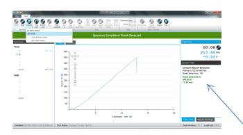
In this example of a tensile strength test we are using the Break Detection feature.
