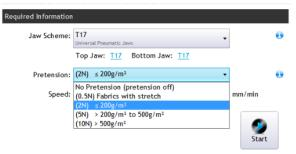
If required, select the required Pretension force, determined by the weight of the fabric (area mass).
