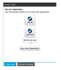
When the position is suitable, click the Save Jaw Separation button.
