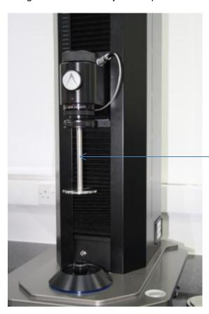
Remove both the top and bottom jaws from the screw thread adaptor.
