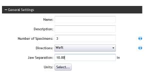
Enter a Jaw Separation (also known as Gauge Length or Gage Length). In this example we are setting a value of 10 inches.
