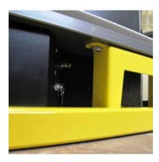
Then unbolt the remaining left and right sides of the bottom frame from the base of the instrument.
