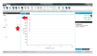
As you proceed through the test specimens you will see the test results accumulating on the left hand side of the **TestWise** screen. For convenience the mean (average) result is also shown.
