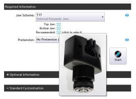
If the mouse is hovered over Bottom Jaw: <u>T17</u> then an image of the jaw is displayed for 5 seconds.
