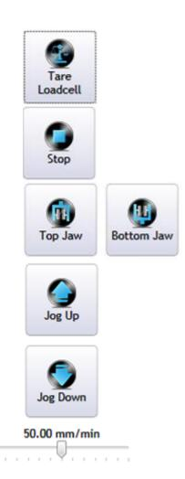
Tares the loadcell reading, resets the force to zero.
