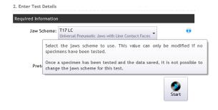
In this example we are setting up to carry out a tensile test according to ISO 13934-1.
