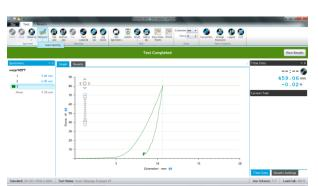
If you need to record any of the manual seam opening measurements, then click Measure-Seam Opening
