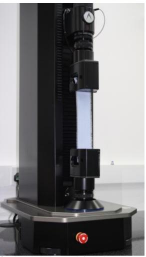
Specimen in the jaws ready for testing
