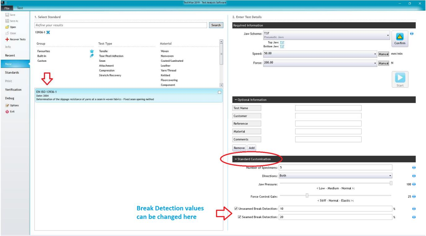
The screenshot shows the 'Enter Test Details' window in TestWise 2019. The 'Standard Customisation' section is highlighted with a red circle. Below it, the 'Unseamed Break Detection' and 'Seamed Break Detection' fields are visible, with values of 10% and 20% respectively. A blue text box with a red arrow points to these fields, stating "Break Detection values can be changed here".
