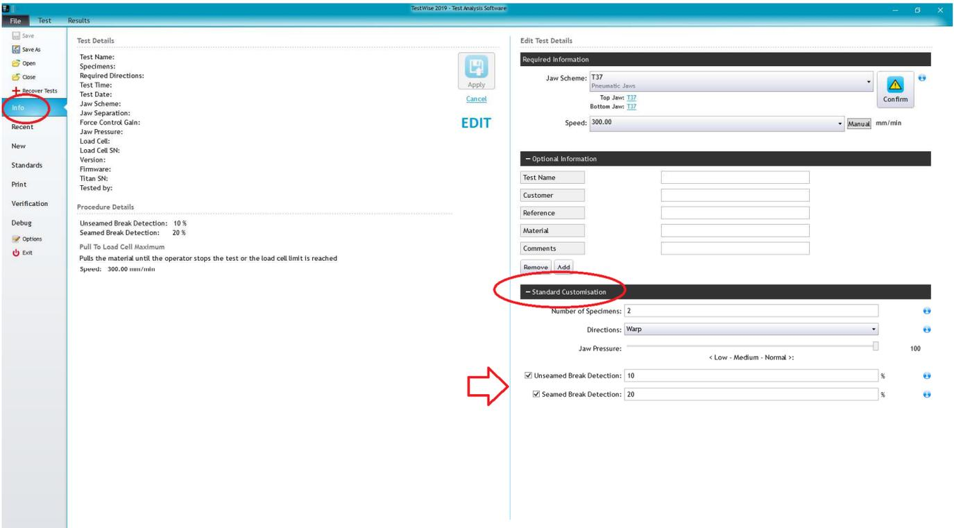
The screenshot shows the 'Edit Test Details' window in TestWise 2019. The 'Info' button in the left sidebar is highlighted with a red circle. A red arrow points to the 'Standard Customisation' section in the 'Edit Test Details' window, which is highlighted with a red circle. Below it, the 'Unseamed Break Detection' and 'Seamed Break Detection' fields are visible, with values of 10% and 20% respectively.
