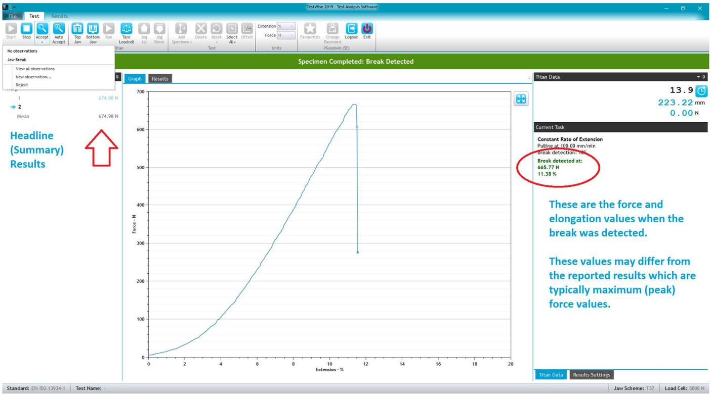
When TestWise detects a break it is saying that the break was detected when the force was 665.77 N and 11.38 % elongation, like co-ordinates on the force/extension curve.
