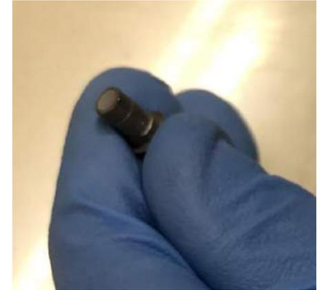
Tip: If you don't have an extra analog to use to protect the interface an alternative is to bury the interface into "Blu Tak" putty before blasting.
