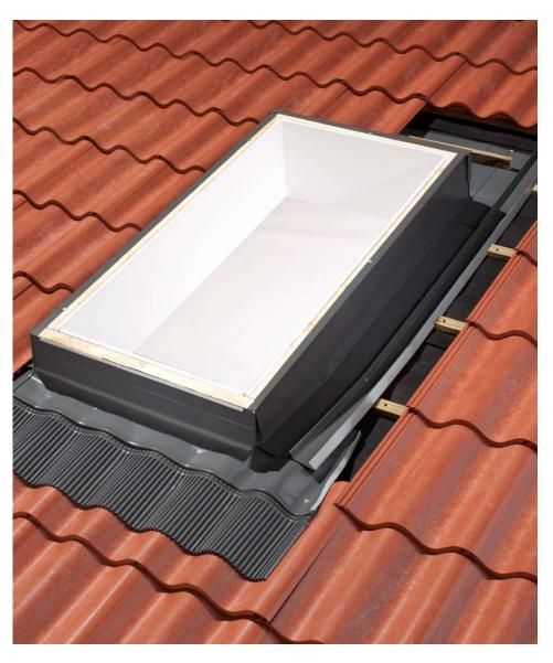
A proven VELUX flashing kit is now made for standard size site-built curbs. ECW tile flashing provides a weathertight seal for standard site built curbs installed on roofs with high profile roofing materials such as concrete or Spanish clay tile.
