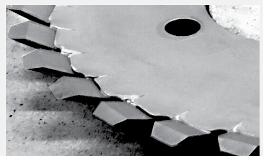
The regular exchange of segments significantly wears down the milling tool. The precise seating of segments is no longer ensured. Further processing becomes more complicated and the quality of the printed products suffers.
