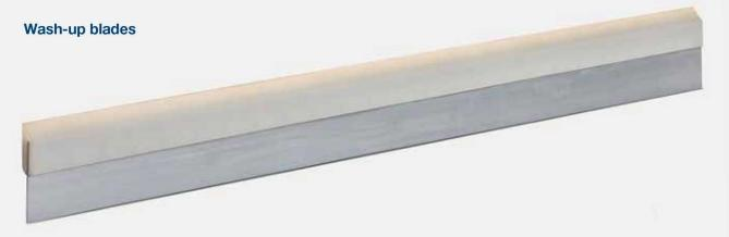
For TKM wash-up blades we generally use Vulkollan® in oder to obtain minimum tolerance deviations. Vulkollan® provides a precise contact zone between wash-up blade and roller and resist swelling. Ink and cleaning agent residues are cleanly scraped off.
