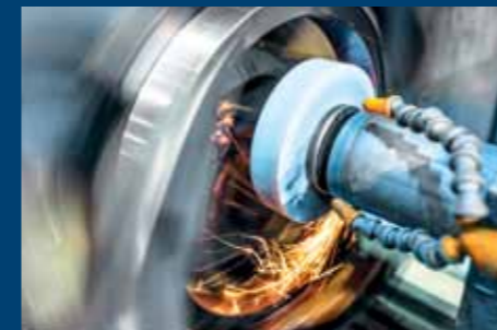
7. Inner Diameter Circular Grinding
