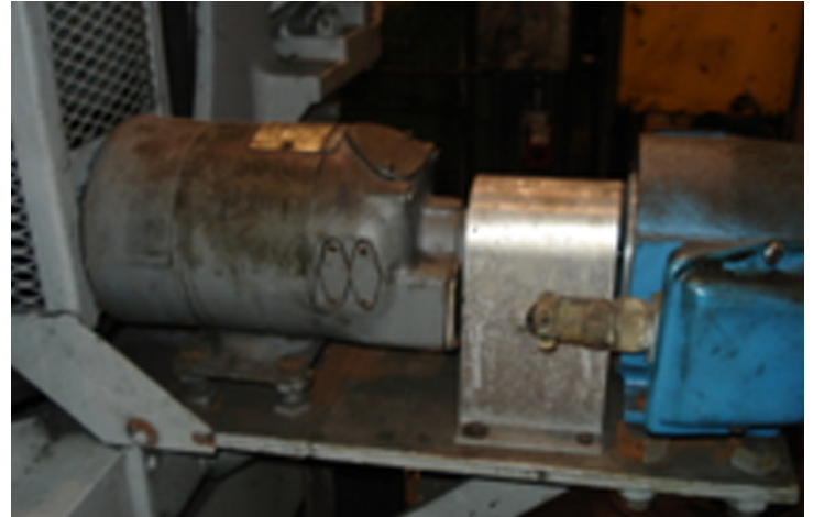
Figure 4A-Tach-Generator/Pulse Generator installation
