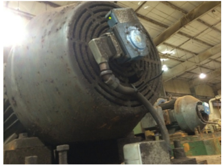
Figure 6 -Encoder mounted on Pickle Line Motor
