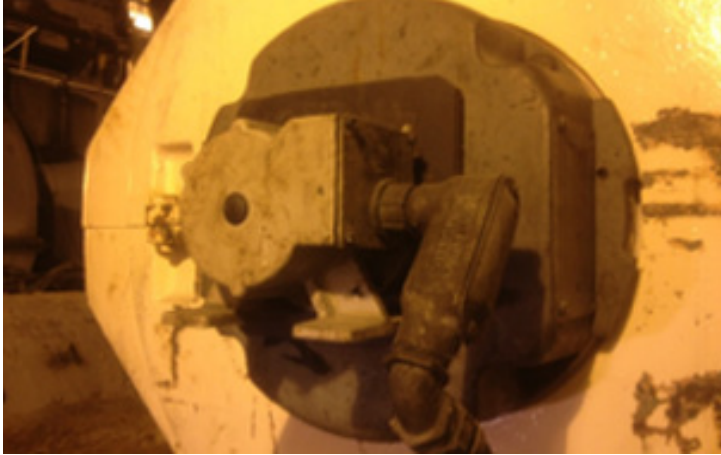
Figure 4-A resolver shown face-mounted and coupled to a motor
