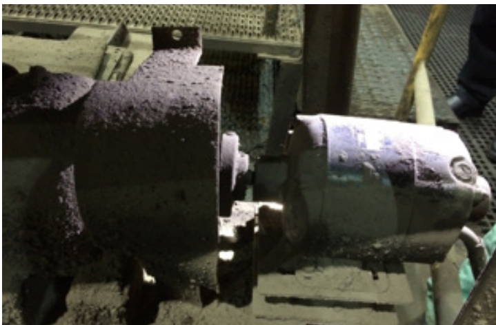
Figure 1-A Selsyn shown foot-mounted and coupled to a metals process
