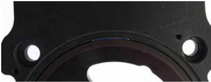
Figure 4- Early Magnetic Encoder, Small Allowable Air-Gap
