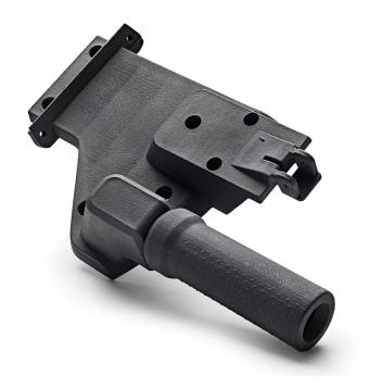
Because the processes is similar to SLS, many of the material options are nylon (polyamide, PA) based. Part properties overall are similar to SLS with slightly higher fatigue resistance. Due to the fusing and detailing agent, HP MJF parts will look matte grey on the exterior and be jet black on the interior. Below are some of the common materials available for HP MJF.
