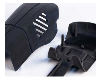
as a finishing step. Because support structure is another material being jetted, there are often indistinct differences on the outside surface of the part which has a tacky feel unless thoroughly treated or scrubbed with an abrasive, like a scotchbrite pad.
