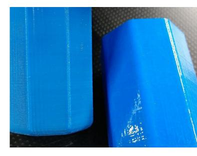
Like machining, vapor smoothing can give parts overall better mechanical properties as well as improved cosmetics. Vapor smoothing can also enable watertight seals on previously porous materials. A downside of vapor smoothing is the denaturing of crisp features, which may appear rounded after the process.
