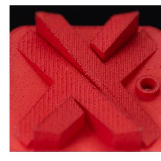
batch due to saturation and exposure. Dyed nylon parts will not pigment full-through, since they are solid in the interior, and will show their natural material color if deeply scratched or cut.
