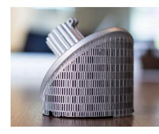
to the level build bed. Since it remains during printing, and after the print, support material can allow the 3D printed part to de-stress while maintaining its intended shape.
