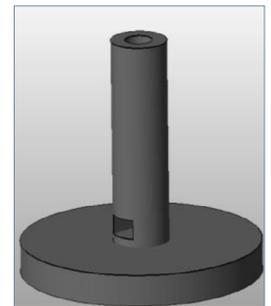
*Model with holes added for removing support material*
