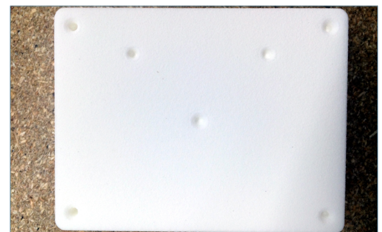
Printed holes that did not successfully resolve
