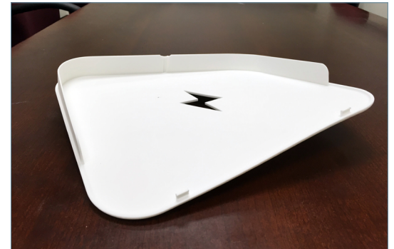
Warping due to uneven cooling
