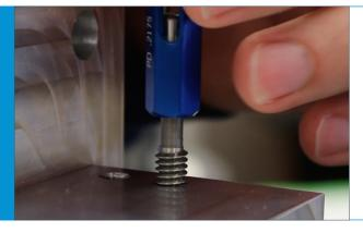
**Check threads** with a calibrated thread gauge.
