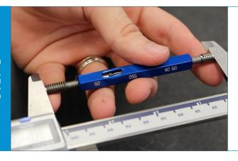
**Check thread depth** with calipers & a mating piece, a go/no-go gauge, or, if the hole is deeper than the gauge allows, an off-the-shelf screw.
