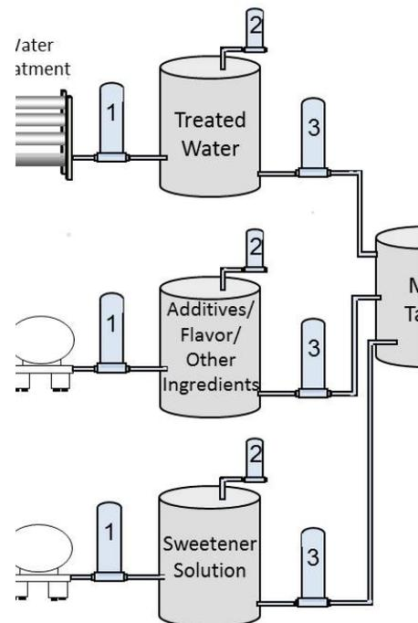
process requires only a reduced bioburden load, then a filter with pore size rating of 0.45, 0.65 or even 0.85 microns might be used, based on what is believed to be in the ingredients. However, if a process requires that an ingredient be “bacteria-free”, then the filter pore size will probably be 0.22 microns or perhaps even 0.10 microns.
