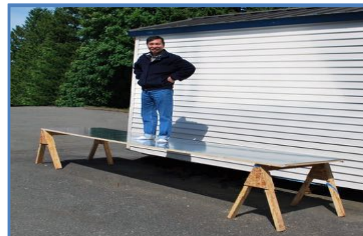
Figure 2 shows the relative stiffness and weight of sandwich panels compared to solid panels
