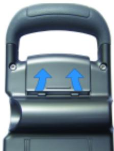
To install the battery, place the battery into the battery compartment with the battery connections lined up. Then place the battery door into back cover, slide the battery door into place and close. The battery door must snap into place.
