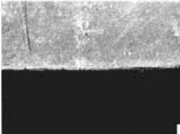
D: Coated Pin after 5000 cycles
