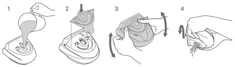
Wash the water chamber, spill guard, tub plate and tub plate seal in warm water, using a mild detergent. Use the yellow cleaning plug to assist in the cleaning process (see steps 1 to 4). Rinse thoroughly in clean water and allow them to dry away from direct sunlight.
