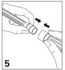
Connect the short tube to the flow generator's air tubing.
