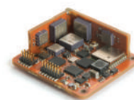
MTi OEM: 37x33x12 mm, 11g, 16-pins header
