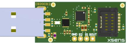
Figure 12: RS232 converter PCB
