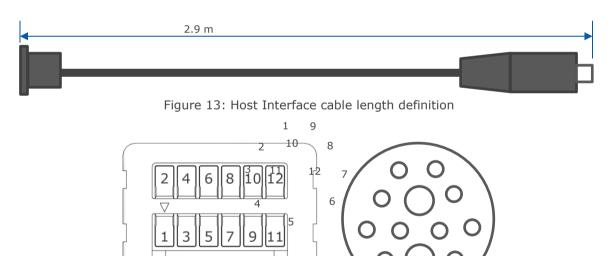
Figure 14: Numbering 12-pin connectors; left Molex (cable entry view), right ODU (solder cup view).
