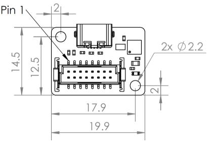
Figure 11: UART to USB converter.
