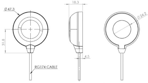
Figure 17: GNSS antenna dimensions (mm)
