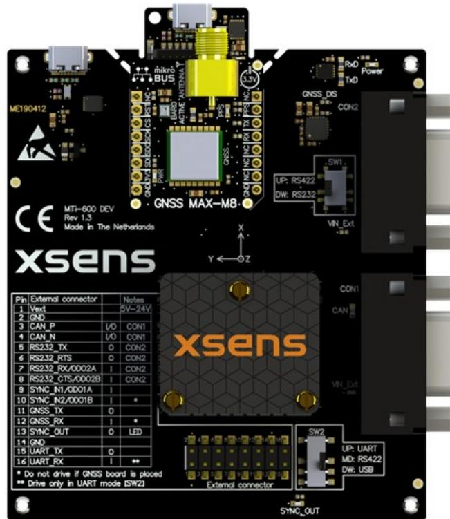
Figure 1: Top view of an assembled MTi-670-DK
