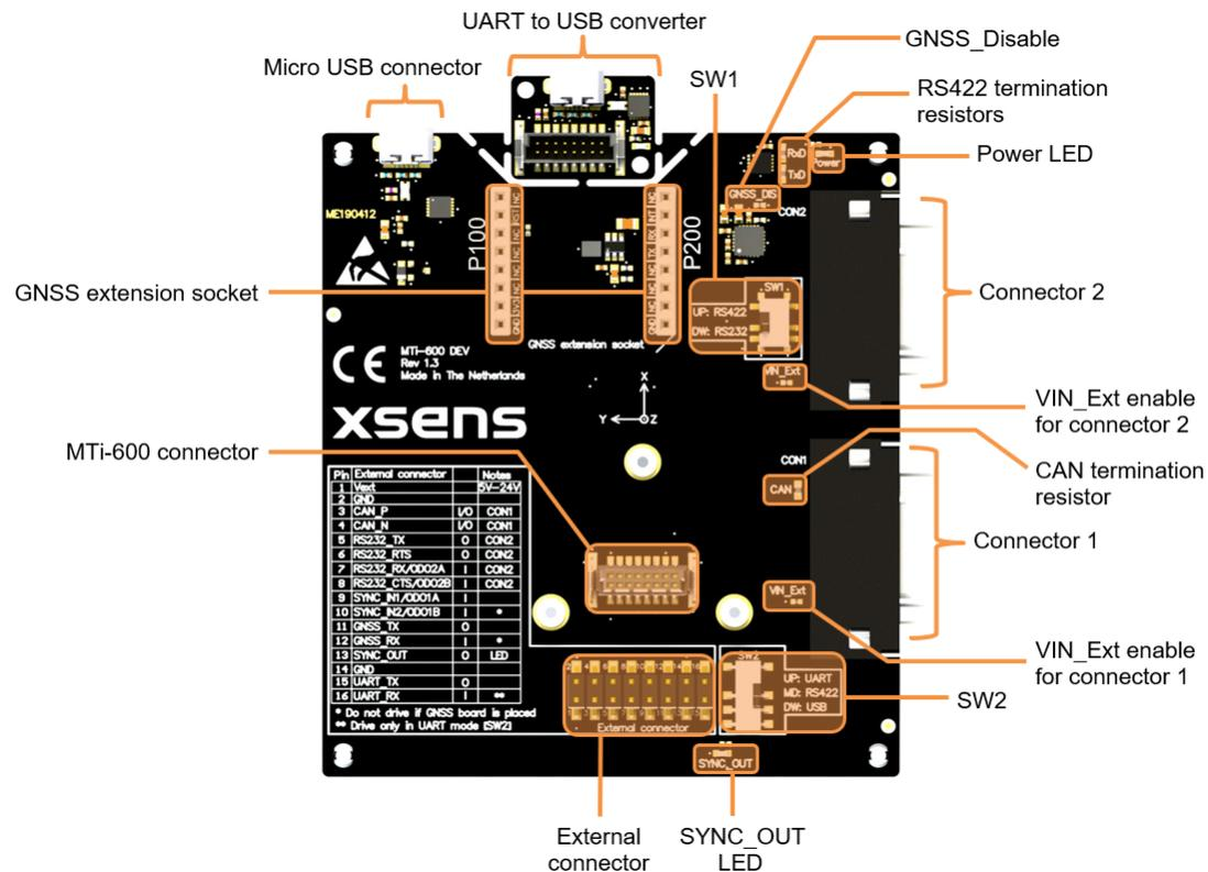
Figure 7: MTi 600-series Development Board overview with connector designators
