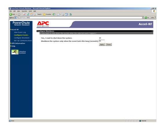
Step 5: Check the "... shut down system" check box. For testing purposes, enter 15 seconds to wait for shutdown after the UPS goes on battery (note: the actual setting should be ~600 seconds, or 10 minutes, after confirmation of shutdown events is complete). Finally, click on Apply to store the settings.
