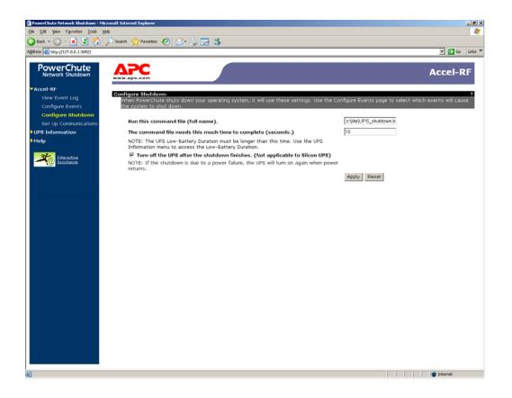
Step 2: Enter the following command file script to run upon shutdown: "C:\LIFE\UPS\_Shutdown.BAT" (note: replace "C:\LIFE" with the application folder if different). For testing purposes, enter 10 seconds for time to complete (note: the actual setting should be ~300 seconds, or 5 minutes, after confirmation of shutdown events is complete). Check the "Turn off UPS..." option. Finally, click on Apply.
