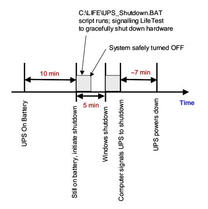
Note that if the main power is restored after the shutdown is initiated, but before the UPS has actually depowered, the UPS Load On/Off must be cycled to clear the shutdown process. Otherwise, the UPS will continue signaling Windows to shutdown after boot up; hence, immediately causing the computer to shutdown again. If main power is restored after the UPS outputs are shut down, then the UPS will automatically reset itself and the power cycling reset is unnecessary.
