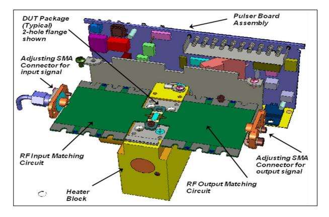
**AARTS RF Device-Under-Test (DUT) Fixture** with DUT & RF input/output circuits installed
