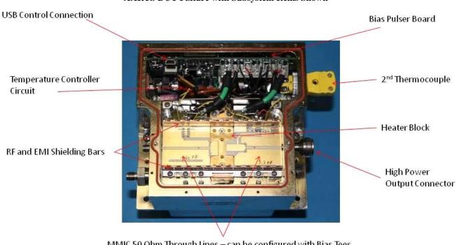
MMIC 50 Ohm Through Lines – can be configured with Bias Tees or Custom Matching circuits. This single board concept (One Input and One Output) can be changed without welding and maintains excellent RF properties.
