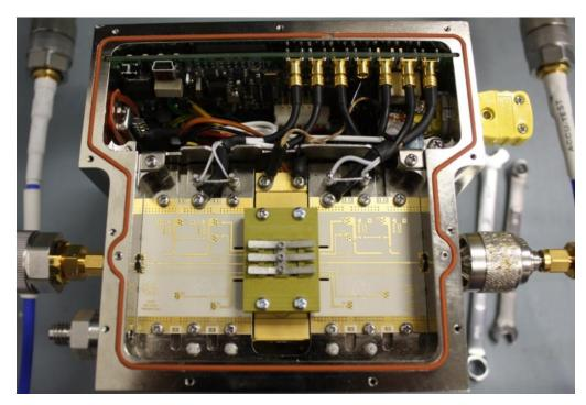
**Bottom Picture: DUT Fixture with MMIC circuits and DUT clamp installed**
