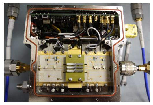
Top Picture: DUT Fixture with Bias-Tee circuits and DUT clamp installed
