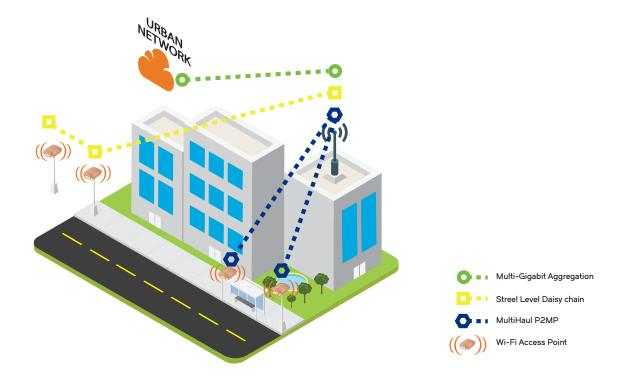
In general, the Siklu mmWave solution provides very high spectrum bands with a lot of available bandwidth. The spectrum bands are short range, 700–2300 ft. for street level and 1–2 Miles for roof tops, which lowers the risk of interference and simplifies RF planning. Lastly, mmWave is unlicensed or lightly licensed, depending on local regulation schemes.
