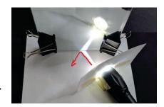
5. Use a protractor to measure the incoming and outgoing angles (the angles between the rays and the mirror line). Record your results in the table below.
