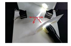
6. Change the angle of the flashlight and repeat the process until you have three sets of angles. Use a new color each time to keep track of each reflection.
