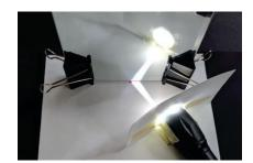
4. Trace the incoming light ray (light going to the mirror) and the outgoing light ray (light reflecting from the mirror): Mark two spots on the paper along each light ray, and then use a ruler to draw a line connecting the dots with the reflection spot.
