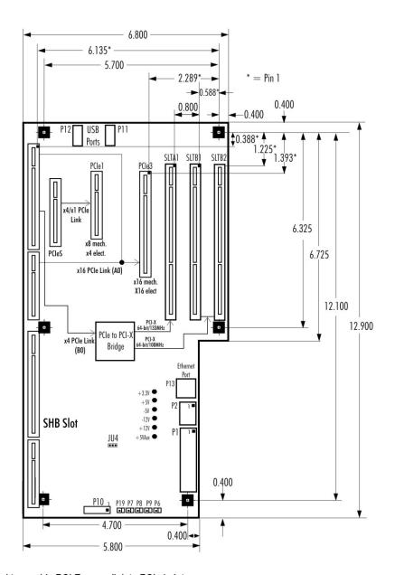
\*IOB31 required to provide PCI Express link to PCIe1 slot \*\*Optional USB, Ethernet connectivity provided by PICMG 1.3 System Host Board. Not all SHBs support this capability. Nominal PCB thickness .062" Connector spacing .800" centers To find the center of a PCI-X/PCI option card connector add 0.150" to the pin 1 location dimension. To find the center of the SHB or a PCI Express option card connector add 0.049" to the pin 1 location dimension. Mounting holes .156" diameter
