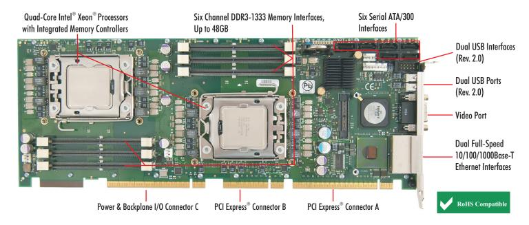
Raising system performance levels while lowering new technology deployment risks and power consumption are key features of Trenton's JXT6966 single board computer. Here's a brief list of the SBC highlights:
