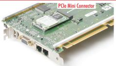
The rear of the THD8141 SHB features a PCIe mini-connector that supports industry standard PCI Express Mini Cards.
