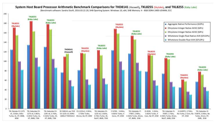
The processor arithmetic benchmark test focuses on the CPU's ability to perform the basic math operations as well as those more advanced computing tasks associated with the AVX instruction set. When comparing exact processor types such as the Intel Xeon E3-1275 v5 (Skylake) to the Intel Xeon E3-1275 v6 (Kaby Lake), the benchmark test results illustrate a noticeable performance improvement when using Kaby Lake especially with the Drystone integer tests.
