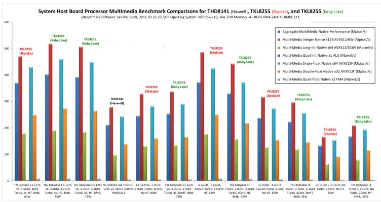
The performance data for multimedia also shows a slight Kaby Lake performance increase over Skylake with equivalent processors. The biggest jump comes when comparing Kaby Lake processor performance to Haswell.
