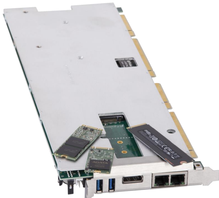
The rear of the TKL8255 and various sizes of M.2 NVMe SSDs.
