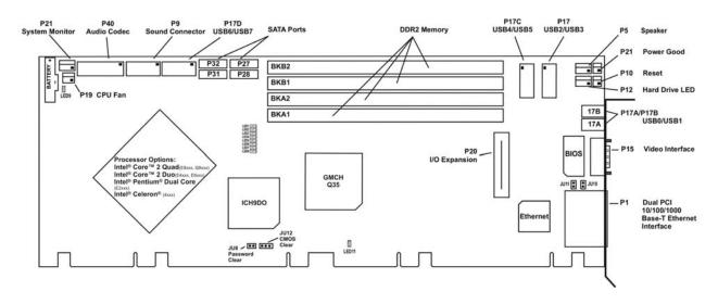
Figure 16 – Trenton TQ9 Connector Layout Drawing
