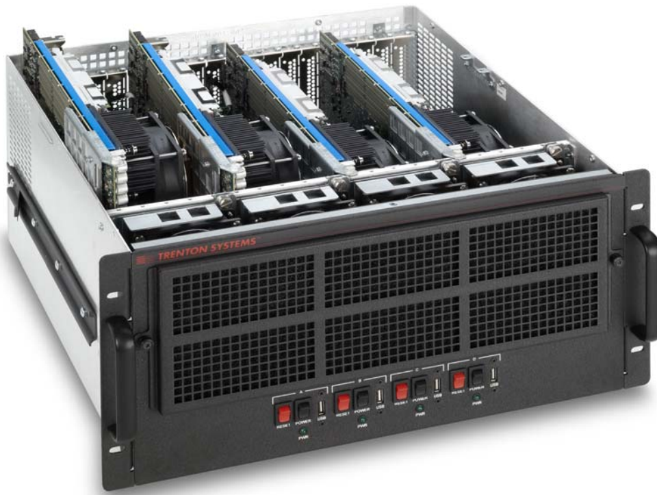
Figure 1. By taking advantage of cluster computing, this lightweight 5U chassis can replace up to sixteen conventional 1U chassis.
