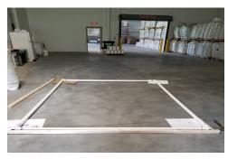
I used 2" PVC for the framing. It was quite easy to assemble the basic framework using, ten-foot sections, "Ts" and 45-degree angles along with end caps. I secured the pieces using PVC Primer and Cement. I then inserted screws into the connections to better secure the joints. I even created a raised tip at the end of each runner to make the structure drag along the pasture more easily.
